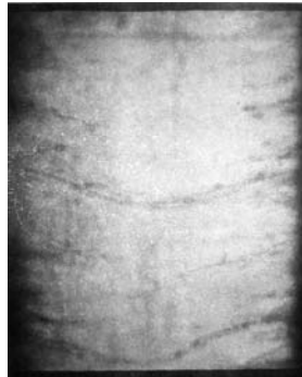
Fig.5 The photo shows that the particles form chains along the field direction, which is perpendicular to the flow direction. The chains jam the liquid flow and are bent. The field direction is perpendicular to the flow direction.
