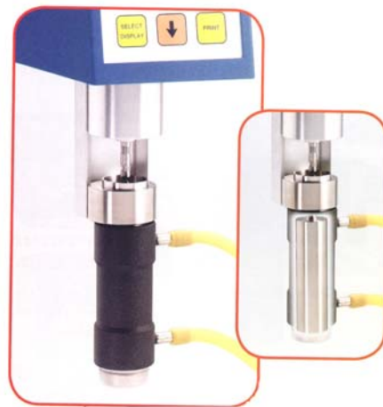
Fig.1 The UL Adapter consists of a precision cylindrical spindle rotating inside an accurately machined tube to measure low viscosity accurately. It also has a water jacket to provide precise temperature control.
